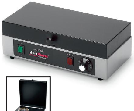
These electric hot plates with thermostatcontrolled bearing heating are especially suited for heating small bearings or small machine parts. The temperature is infinitely adjustable from 50°C to 200°C.
