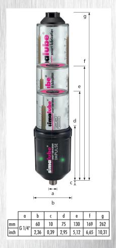
The simalube® IMPULSE ensures reliable lubrication in situations with high counterpressure and long lubrication lines. Together with the automatic simalube lubricators, this pressure booster pumps greases and oils at up to 145 psi and 0.02 fl. oz. per impulse to the required lubrication point. The LED display of the intelligent pressure booster provides information continously about the current operating condition, and flashes green when the device is functioning correctly.
