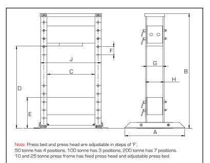
Press Capacity Frame dimensions in mm Range tonnes А В С D (min) D (max) E (min) E (max) F G Н J HPF1000 10 742 1448 508 1258 260 1010 150 152 660 \_ HPF2500 25 742 1448 508 1258 260 1010 150 -152 660 HPF5000 50 2055 800 1140 395 815 140 1000 1000 1560 258 298 100 1370 550 1240 HPF10000 1000 1980 1000 1090 830 140 338 388 HPF20000 200 1200 2500 1250 1815 2115 610 1510 150 330 410 1750
