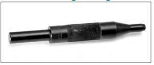
These tools are designed to flare or bell a projecting tube end. They are usually supplied with a shank .680" diameter x  $2^{3}/_{8}$ " long. Details of the tube end conditions to be supplied with your enquiry.
