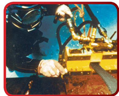
Wachs Trav-L-Cutter is versatile and adaptable to Subsea operation
