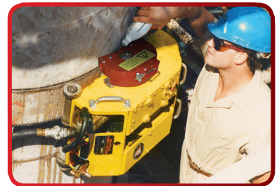
Highly versatile, the Trav-L-Cutter can cut vertically, horizontally or anything in between
