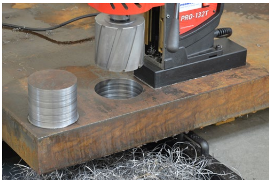
Milling capacity up to 130 mm (5") Max depth of cut up to 100 mm (4")
