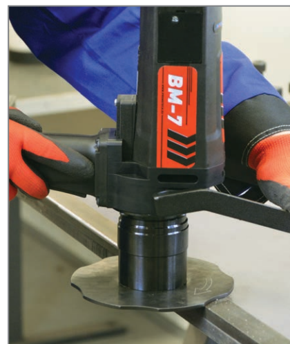
Straight edge beveling with radius
