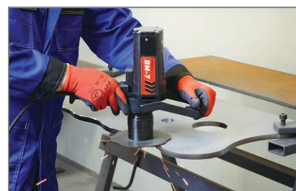
Arched edge beveling with radius
